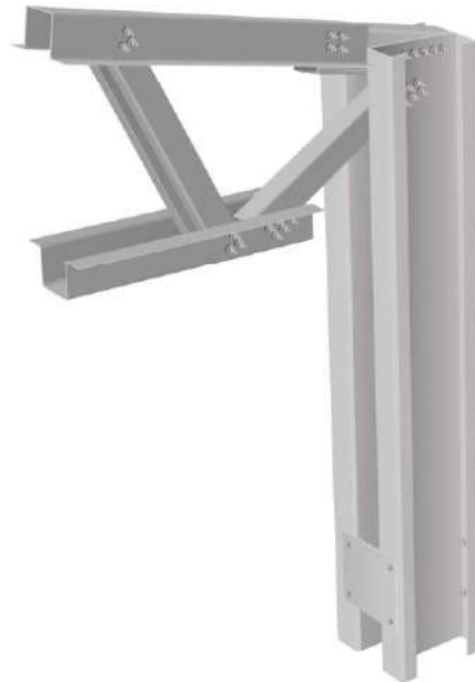
HINGED CONNECTION TO REINFORCED CONCRETE COLUMN
