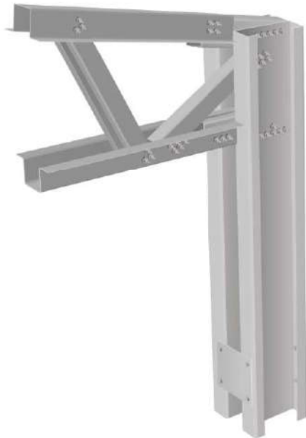
HINGED CONNECTION TO REINFORCED CONCRETE COLUMN
